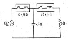
21. Determine the components of the load impedance Z<sub>L</sub> that will develop maximum power:
